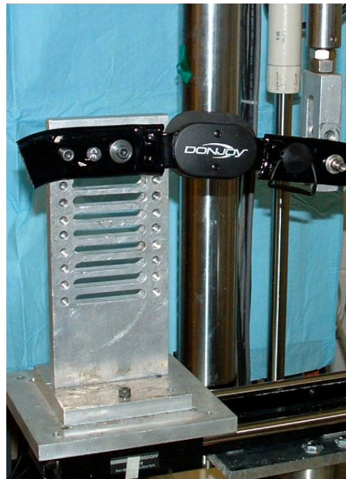
Figure 3: Extension-Locking Hinge Mechanism Testing
